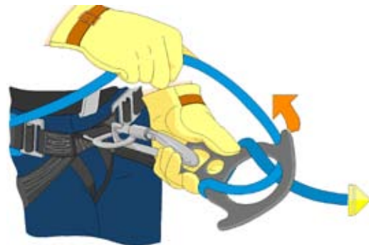
Figure 2:95 Pull the Running End of the Rope
