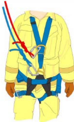
Figure 2:55 Main line with chest Belay/Safety line attachment
