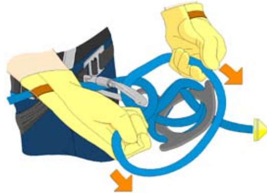
Figure 2:100 Pass the Loop over the Top
