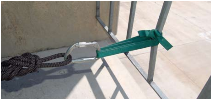
Figure 2:38 Wrap Three Pull Two Sling around a rusty railing.
