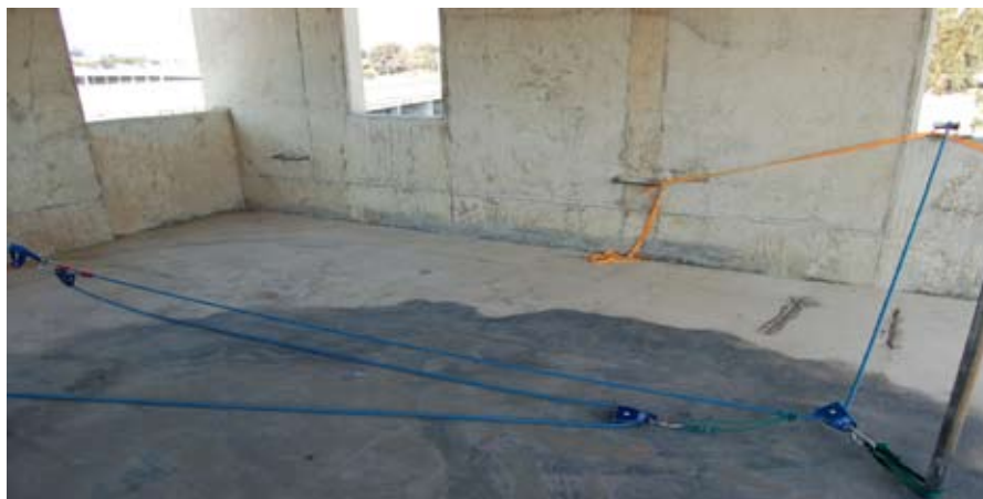
Figure 2:118 RPM 3:1 MA system with change of direction pulley
