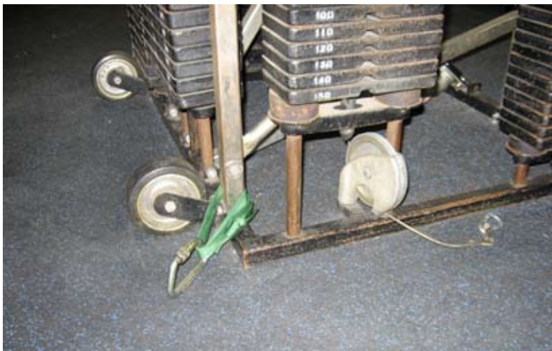
Figure 2:37 Multiloop Sling around a weight machine.
