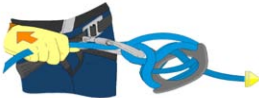
Figure 2:99 Pull the Running End to Tighten
