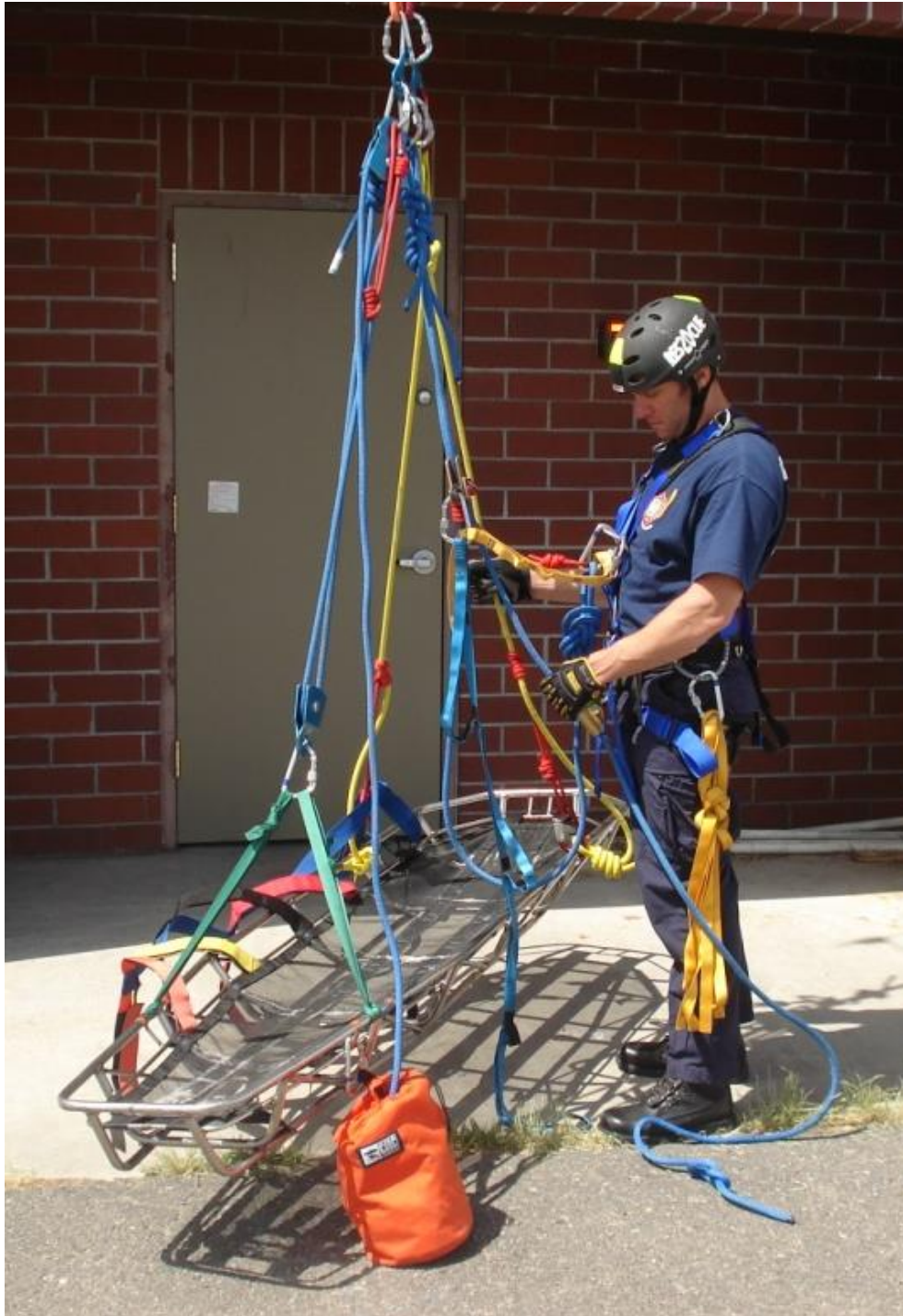
Figure 15-10. The rescuer is prepared for a litter scoop. He is attached to the system as seen before but carries webbing to use as interior lashing to secure the patient into the litter. The top half of the litter is rigged as before but the bottom half litter pre-rig is replaced with a ladder rig and prusik at the top pulley. Velcro straps have been pre-positioned on the litter ready to be used as exterior lashing to secure the patient into the litter.
