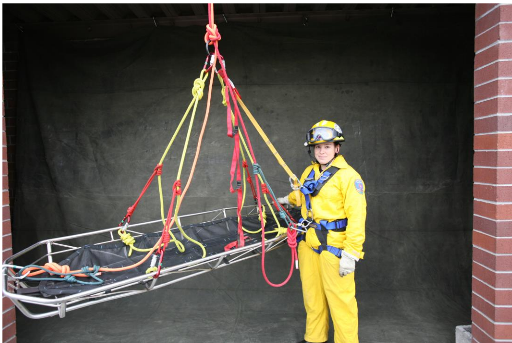
Figure 15-19. The rescuer and litter are attached as seen above. One longtail is attached to the rescuer and the other longtail is attached to the head of the stokes. System redundancy for the rescuer and patient is achieved.
