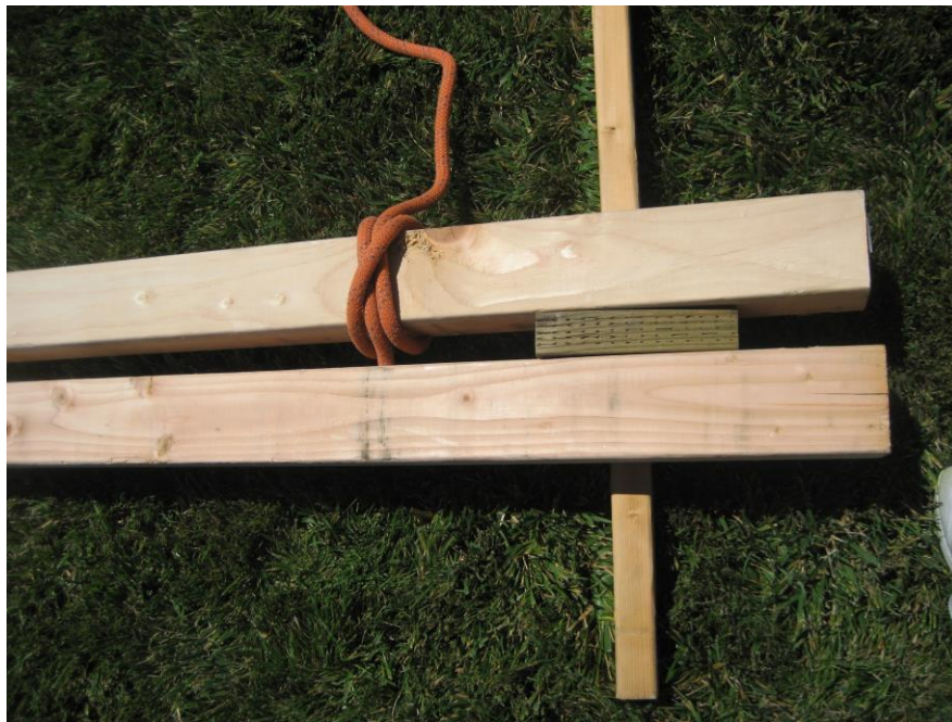
Figure 16-5. Clove hitch on one leg.
