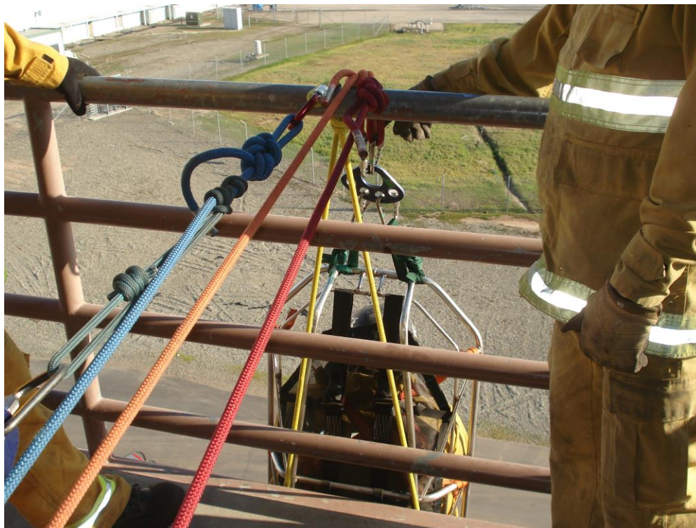
Figure 15-8. The "V" Strap is disconnected from the anchor plate and connected to a separate mechanical advantage system.
