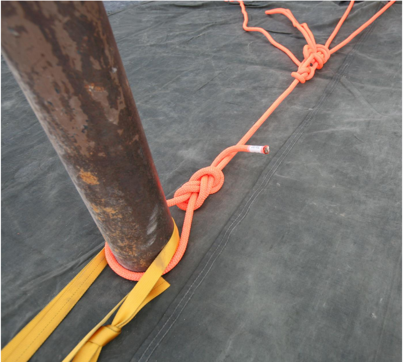
Figure 4-3. Back tied anchor.
