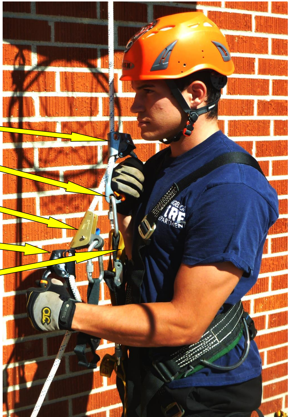
Figure 12-1. Ascending Attachment Points
