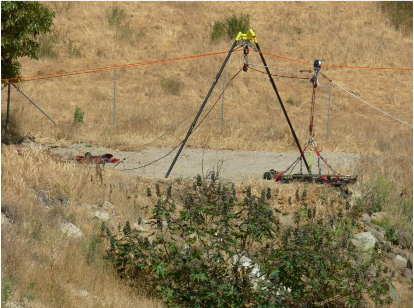
Figure 16-1. Artificial High Directional.
