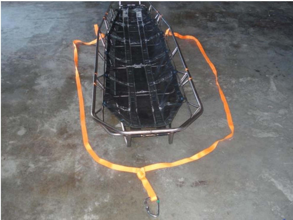
Figure 15-6. An alternate method for the "V" Strap is to use a 20' piece of webbing.
