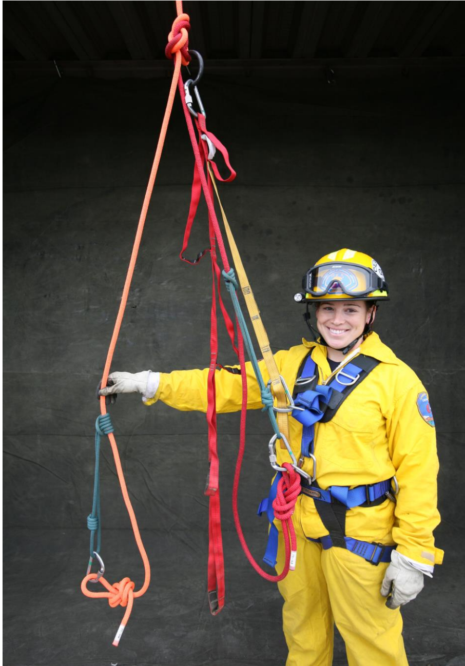
Figure 15-17. A longtail bowline is tied in the main line and the belay line with a steel ring in the knot and an etrier connected to the steel ring. The rescuer is attached to one line and the etrier. The other line is used to attach the victim to the system.
