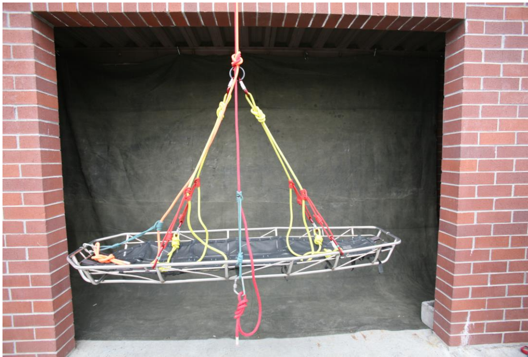
Figure 15-18. The litter pre-rig is attached to the Steel Ring.
