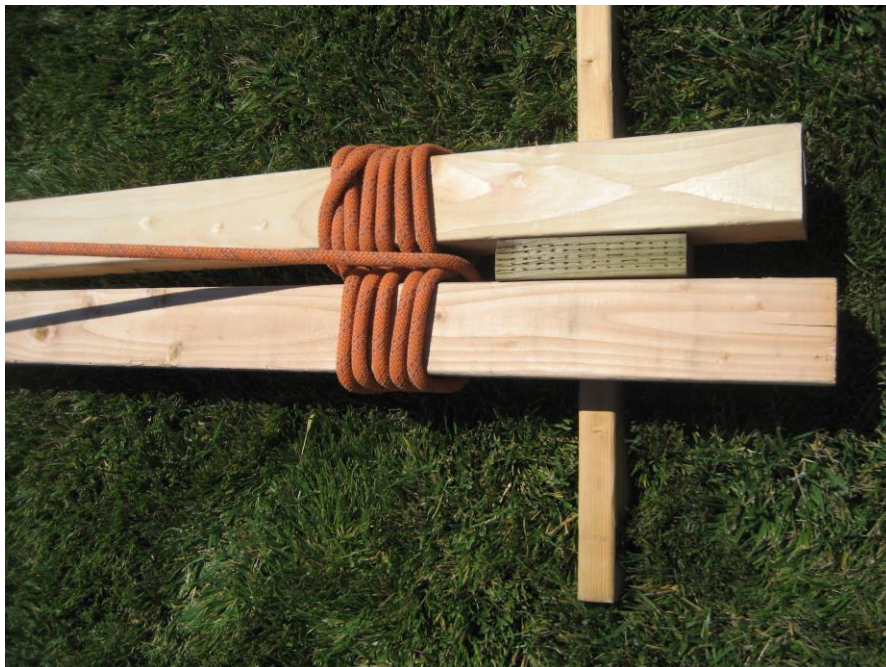
Figure 16-6. Wrapping and frapping.
